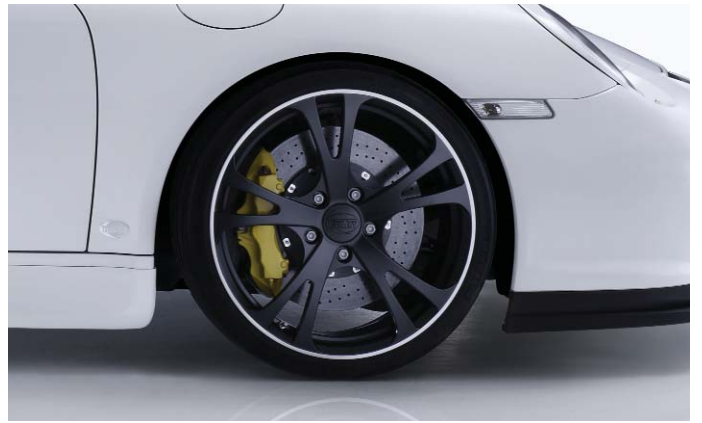
TECHART Formula III forged Leichtmetallrad in mattschwarz/weiß lackiert TECHART Formula III forged light alloy wheel painted in Matt Black/White
