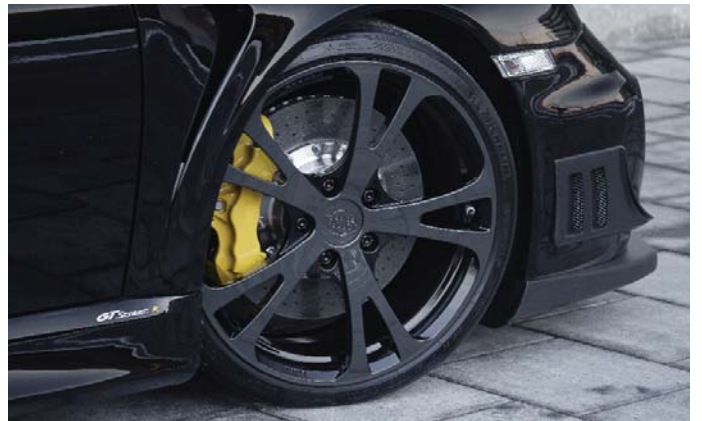
TECHART Formula III forged Leichtmetallrad zweifarbig phantomgrau/schwarz lackiert TECHART Formula III forged light alloy wheel painted in Phantom Grey/Black bicolor
